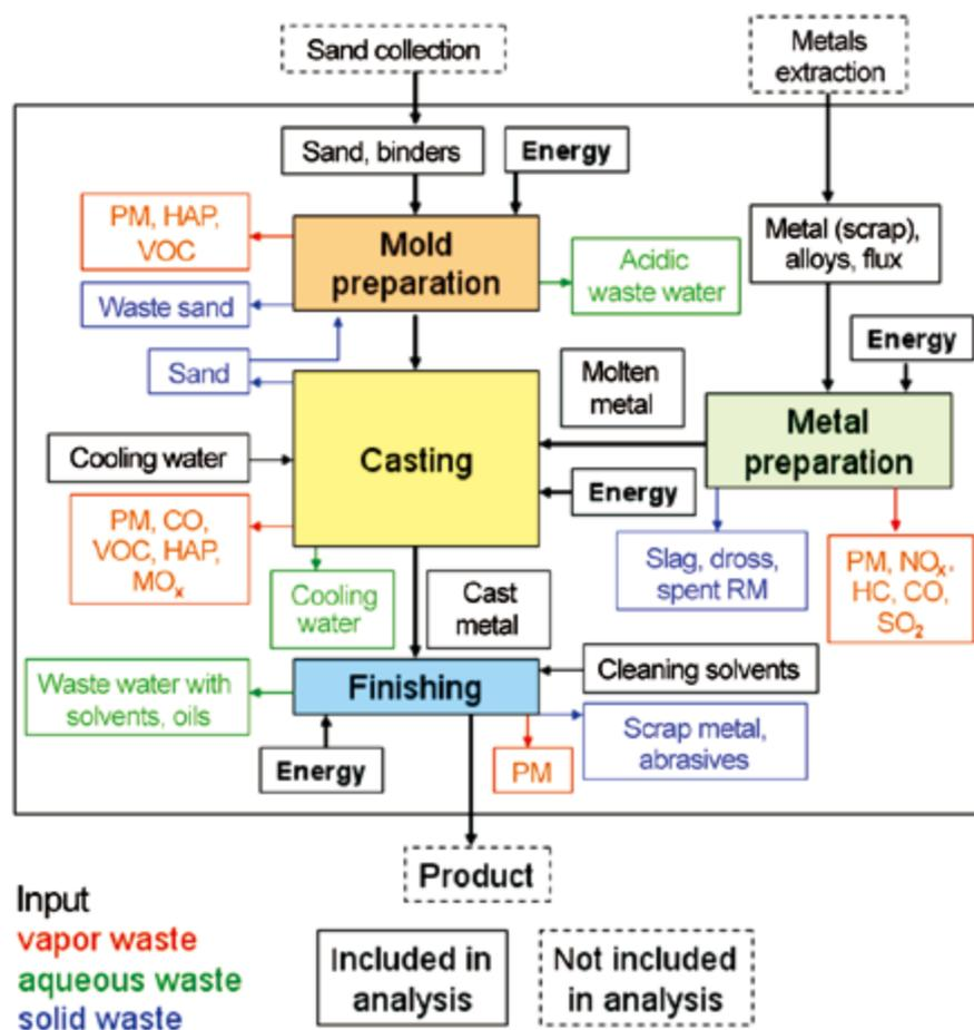
Fig. 1: Example of foundry system waste streams [2]
