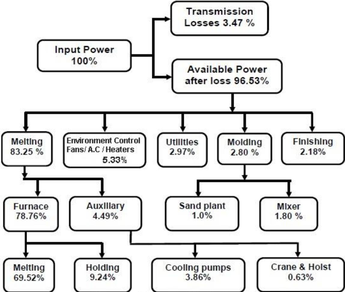
Figure1. Power distribution tree of Foundry
