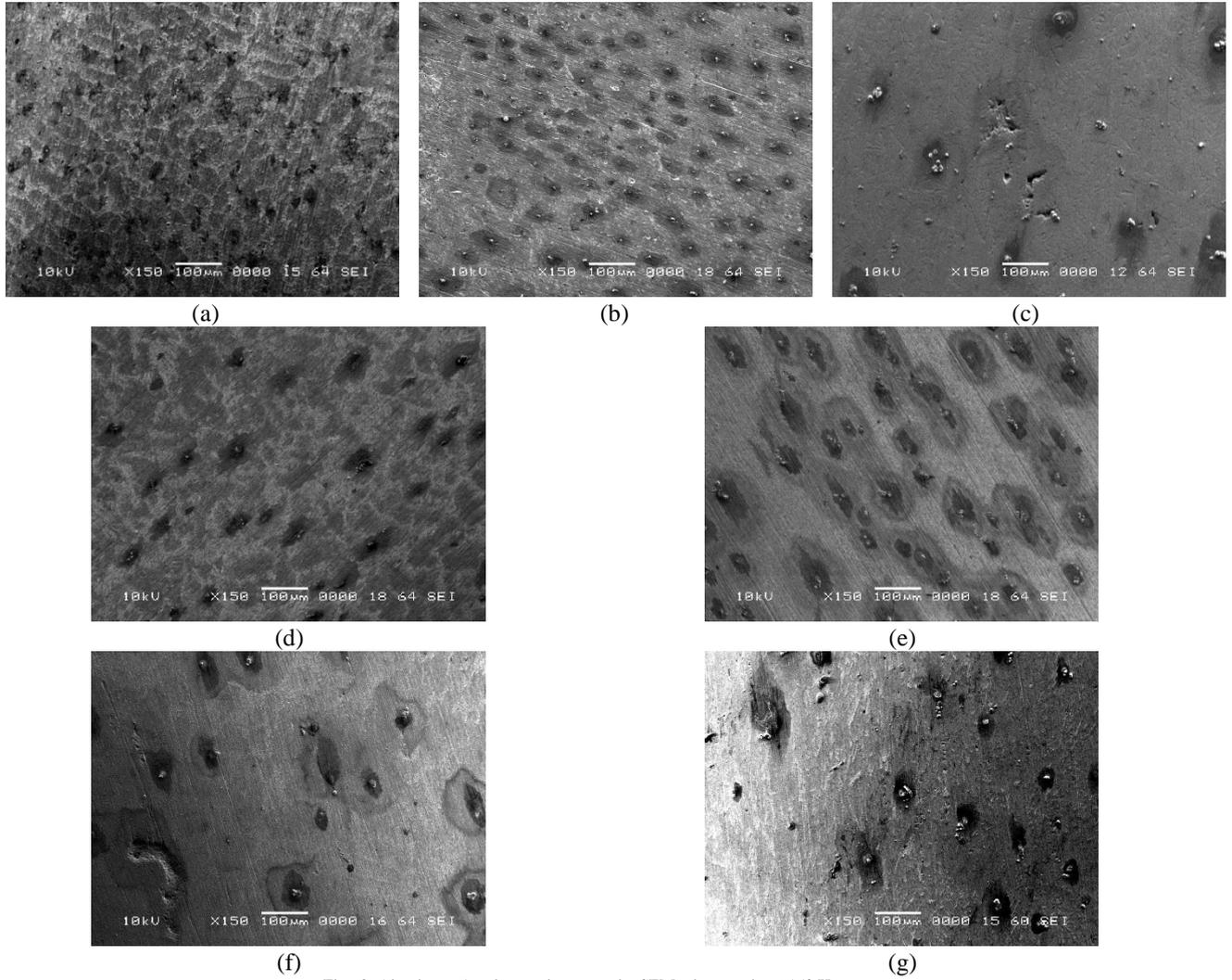
Fig. 3: Aluminum-5% zinc- ceria composite SEM micrographs at 150 X
