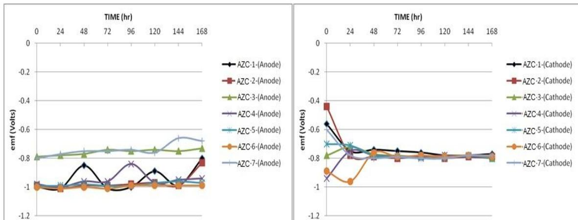
Fig. 6: Time vs. CCP graph [AZC-1 to AZC-7 (anode+cathode)]
