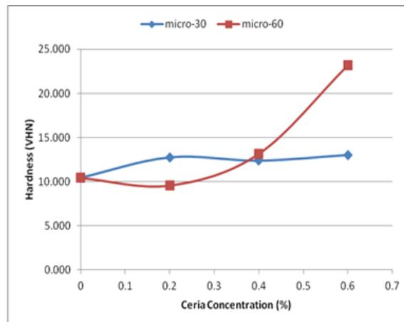
Fig. 4: Aluminum-5% zinc- ceria composite Hardness
