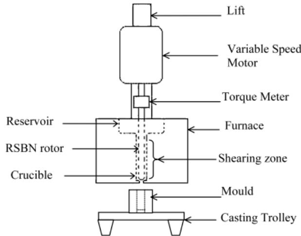
Fig. 1: Schematic diagram of stir casting device
