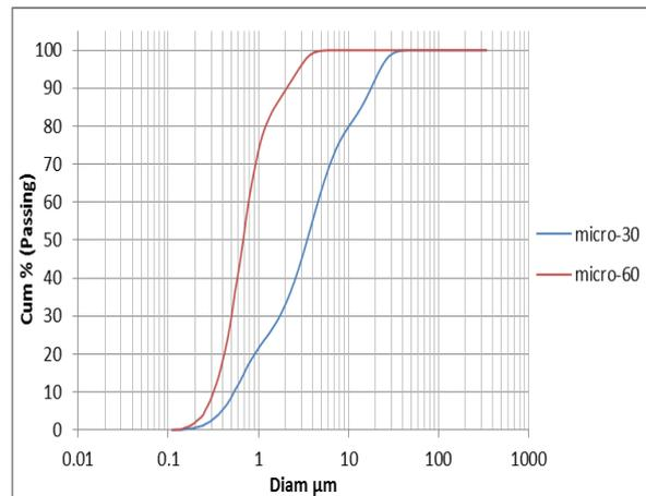
Fig. 2: Cumulative particle distribution of 30min and 60 min ground sample
