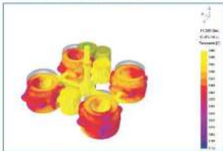
FIGURE 7. Model 3Ding showing temperature distribution.
