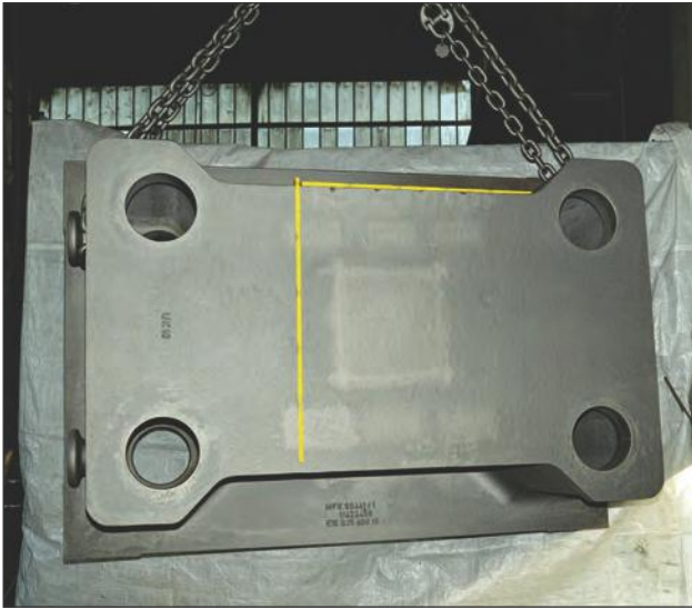
Fig.1 Highest surface quality: In this cross-member for a pressing machine made of GJS 400-18, the entire surface (100 per cent) undergoes magnetic particle inspection
