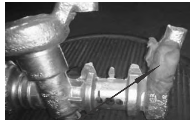
Fig 8: Side riser height was increased, for improving feeding. The Head which force the hot metal into the shrinkage area
