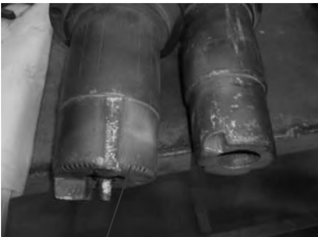
Fig 13 : Aluminium metal pick-up on the 120 dia core, noticed after removing the die coat
