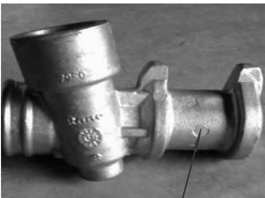
Fig1: Critical bore is 29 dia, inside
