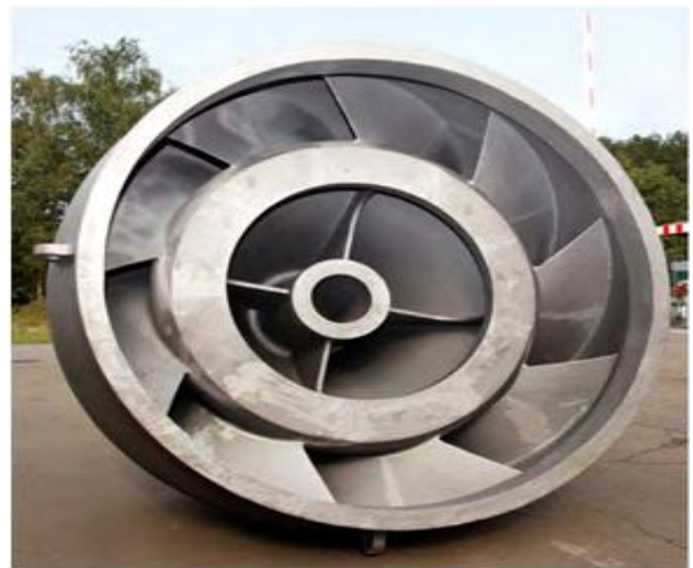
Guide vane housing made of GJS 400, Weight: seven tonnes
