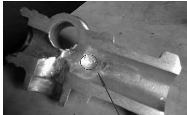
Fig 2: Shrinkage in the 29 dia bore
