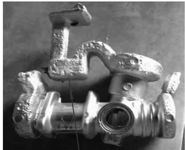
Fig 7: Modified running system with 1:4:2 ratio, single pouring Basin was provided
