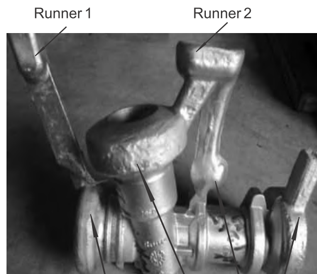
Fig:3. Full shot casting with Risers & Runners and gate entries for metal into the cavity
