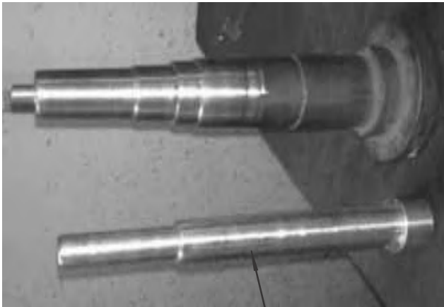
Fig 9: Side core with Long copper chill, which was inserted with tight fit, inside the core, by making a long bore.
